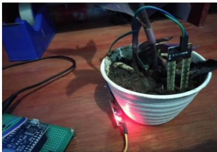
Gambar 9. Pengujian Sensor Soil Moisture
